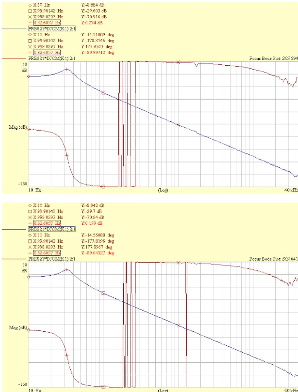
Figure 6: Focus tracking bode plots for Blu-ray OPU
