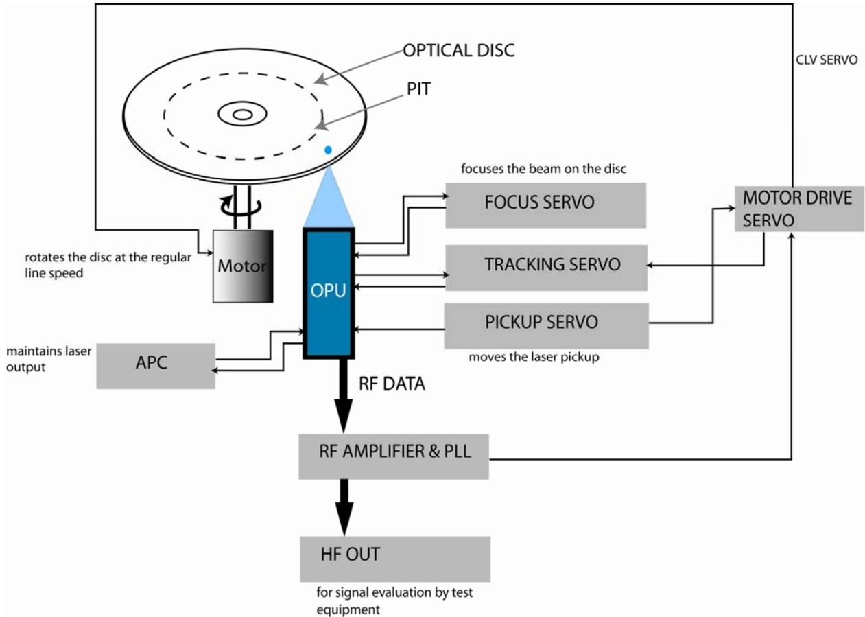
**Figure 5: block diagram of drive**
