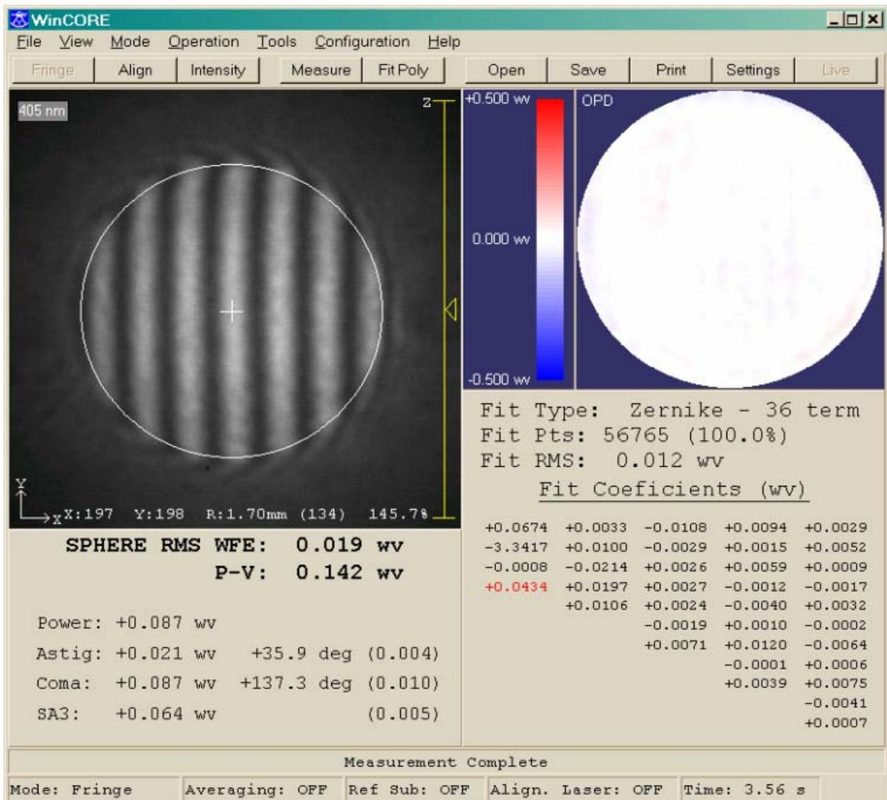
**Figure 3: Beam only 19 milliwaves RMS**
