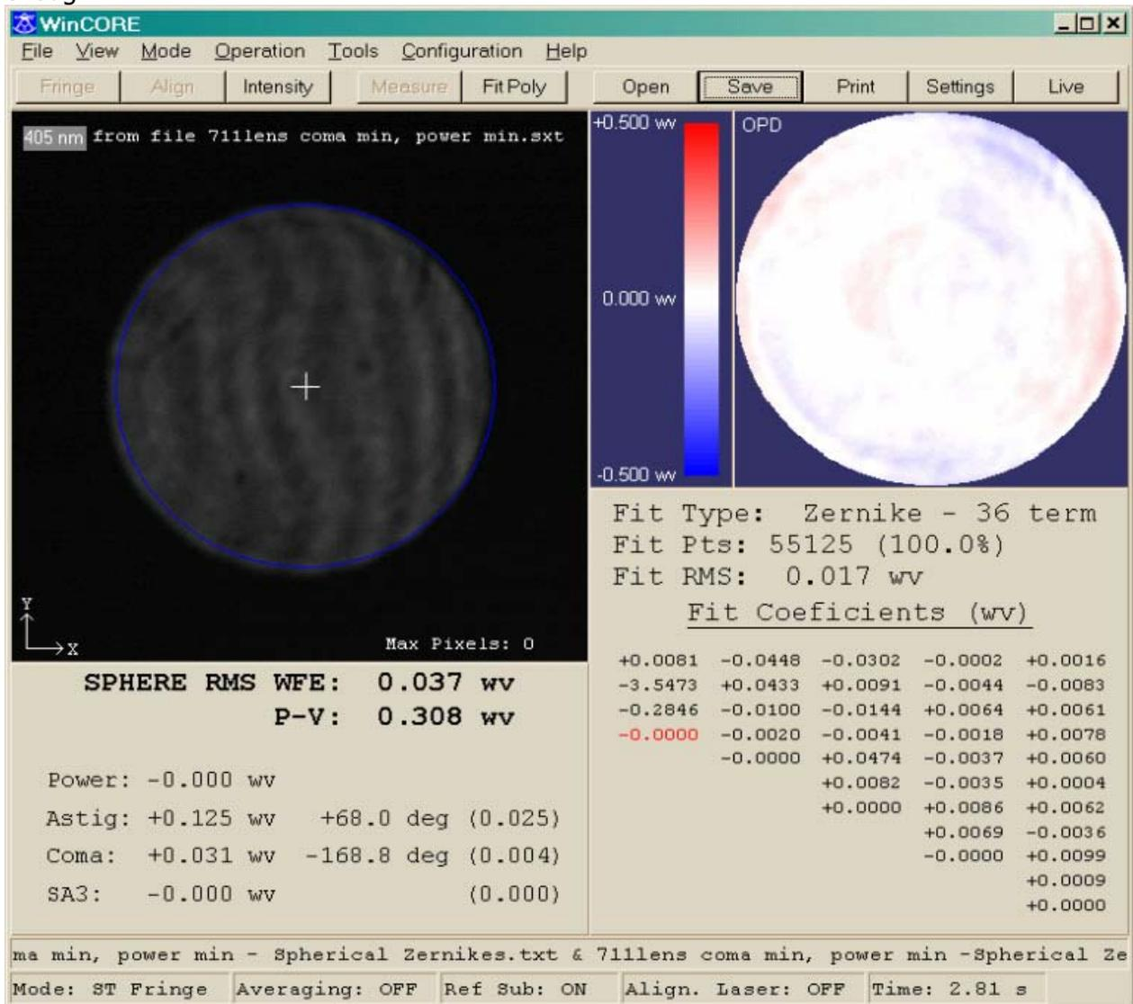
Figure 4: lens only 37 milliwaves RMS
