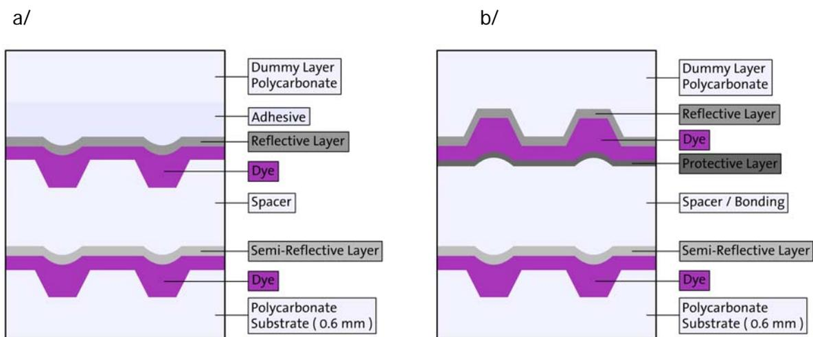
Figure 2. Schematic presentation of 'simple' (a) and 'reversed' (b) recording stack design for DVD+R DL discs
