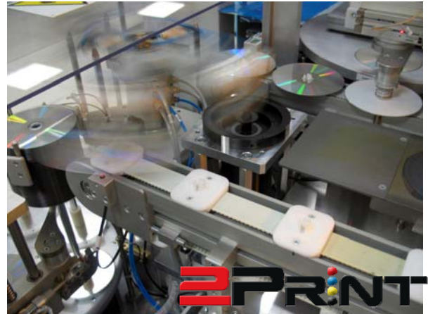
Figure 1: DaTARIUS Ident Code Inspector in Tapematic's 2PRINT
